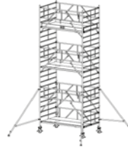
Working height: 7.30 m Platform height: 5.30 m Scaffold height: 6.40 m
